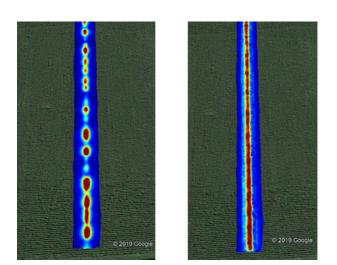
Figure 3. Resulting magnetic maps of the previous inspected area. The two maps rely on the same dataset but treated with different algorithms.
